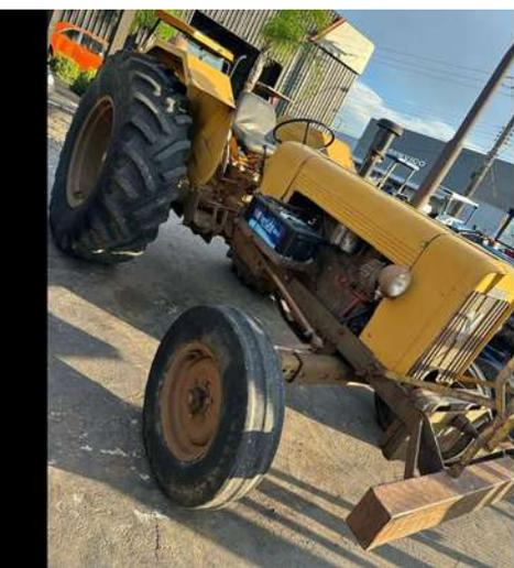
TRATOR COM MOTOR MWM 4 CILINDROS DE 78 CV DE POTÊNCIA E BOMBA INJETORA BOCH
